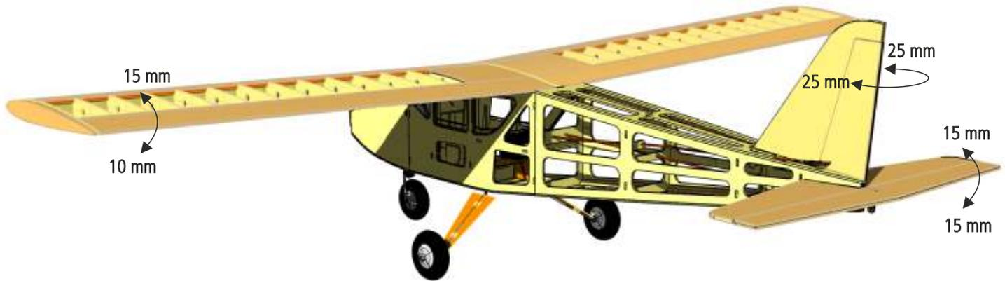
**Electric power:** Install motor and connect ESC and servos to receiver. Do not fit the propeller yet. Connect battery to ESC and adjust control throws of servos. Secure battery on battery tray with velcro or similar and balance model. The centre of gravity is located 65 mm behind the wing's leading edge. If possible, adjust centre of gravity by repositioning battery.
